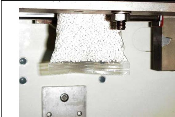
**Figure 8c: Strong deformation of the sealing area**
